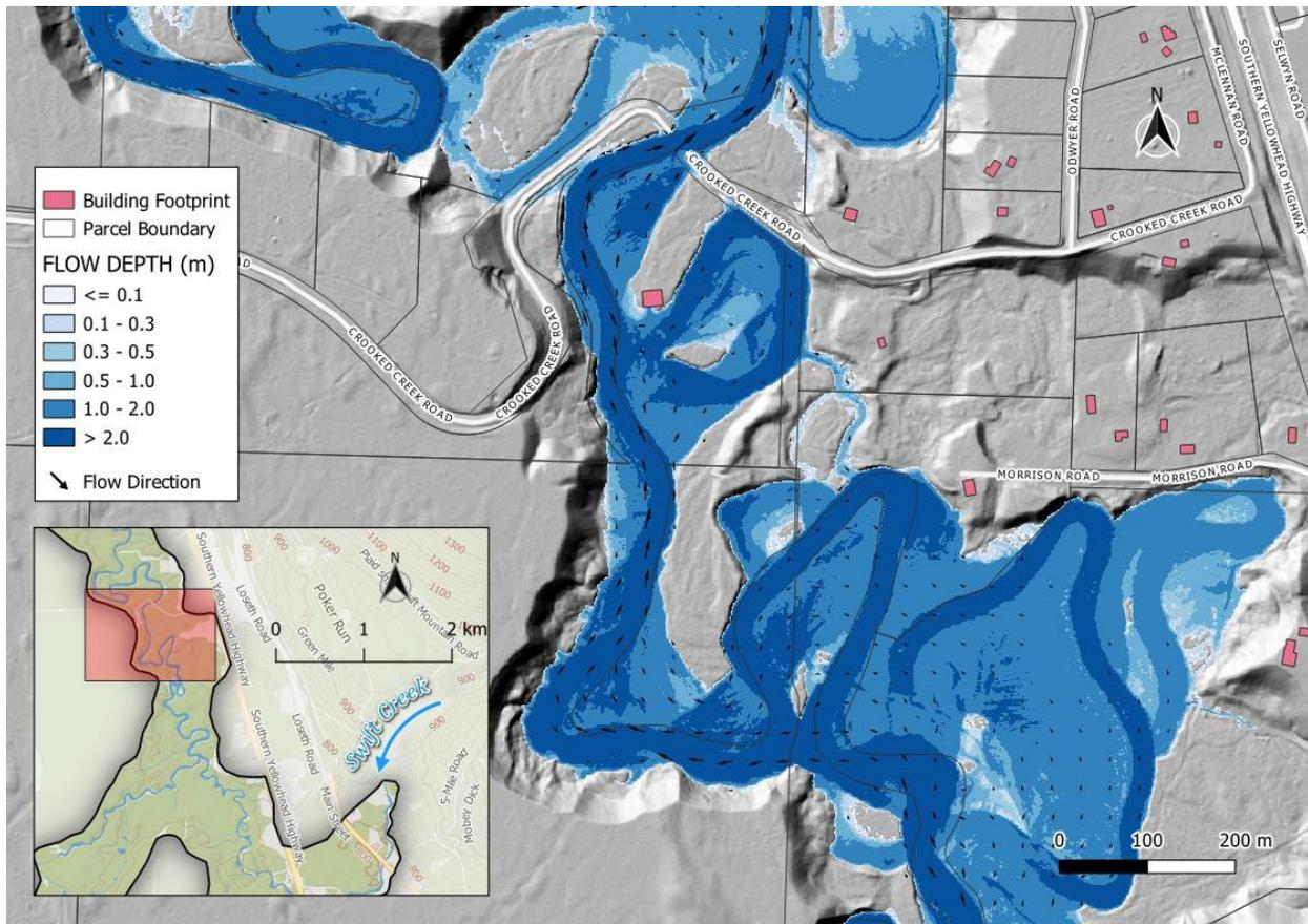
**Figure E-38 Modelled climate-adjusted 200-year (0.5% AEP) McLennan River flood depth in the vicinity of Crooked Creek Road, overlaid on the DEM (hillshade). Arrow size is proportional to flow velocity. Building footprints from Microsoft (2023) database (additional buildings likely exist). Parcel boundaries from BC Assessment (2023).**
