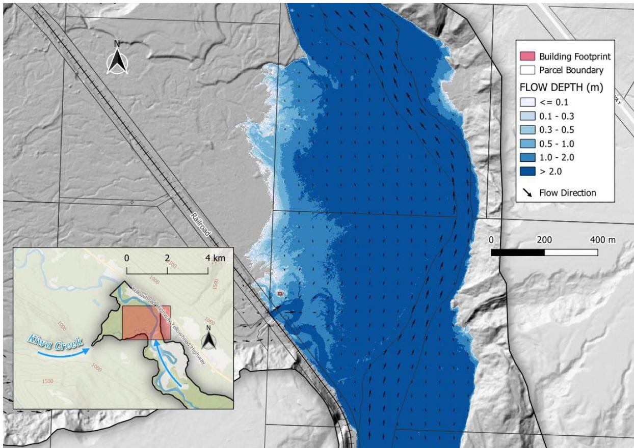
**Figure E-35 Modelled climate-adjusted 200-year (0.5% AEP) flood depth at the confluence of Fraser River and Kiwa Creek, overlaid on the DEM (hillshade). Arrow size is proportional to flow velocity. Building footprints from Microsoft (2023) database (additional buildings likely exist). Parcel boundaries from BC Assessment (2023). The building footprint shown is located on a terrain high point and is not expected to be flooded.**
