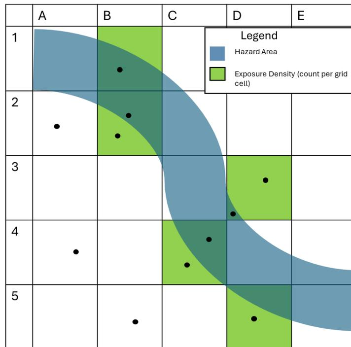
**Figure H-2 Schematic of the hazard exposure calculation logic for point-based valued assets.**
