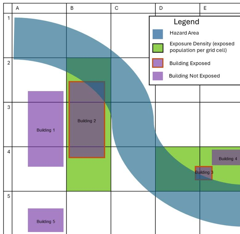
**Figure H-5 Schematic of the hazard exposure calculation logic for population.**
