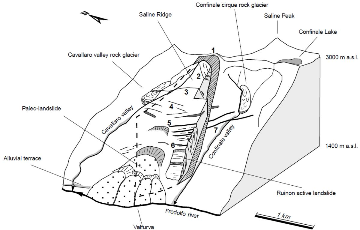
**Figure G-5 Three-dimensional model of mountain slope deformation (Agliardi et al., 2001).**
