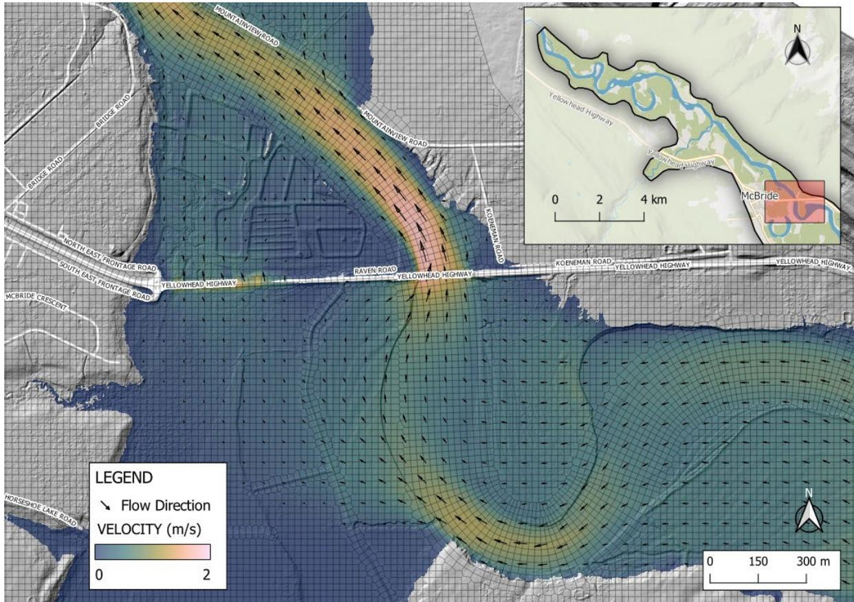
**Figure E-14** Example of the mesh developed for the Fraser River at McBride HEC-RAS model in the vicinity of McBride Bridge. Modelled flow velocities for the stationary 200-year flood event are overlaid on the DEM (hillshade). Arrow size is proportional to flow velocity.
