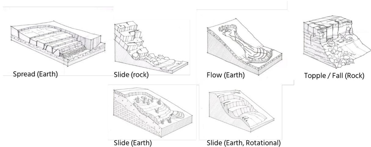
**Figure 4-4 Schematic examples (not exhaustive) of landslide movement types, adapted from Hungr et al. (2014).**
