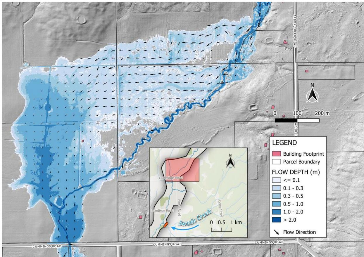
**Figure E-24 Modelled climate-adjusted 200-year (0.5% AEP) Tabor Creek flood depth in the vicinity of Cummings Road, overlaid on the DEM (hillshade). Arrow size is proportional to flow velocity. Building footprints from Microsoft (2023) database (additional buildings likely exist). Parcel boundaries from BC Assessment (2023).**
