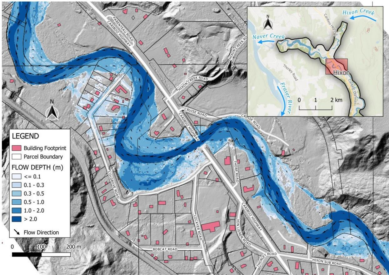
**Figure E-26 Modelled climate-adjusted 200-year (0.5% AEP) Naver Creek flood depth in the vicinity of the Canyon Creek bridge (Cariboo Highway), overlaid on the DEM (hillshade). Arrow size is proportional to flow velocity. Building footprints from Microsoft (2023) database (additional buildings may exist). Parcel boundaries from BC Assessment (2023).**
