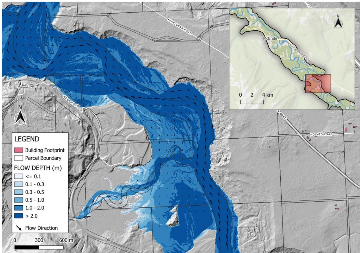
**Figure E-31 Modelled climate-adjusted 200-year (0.5% AEP) Fraser River flood depth in the vicinity of Castle Creek, overlaid on the DEM (hillshade). Arrow size is proportional to flow velocity. Building footprints from Microsoft (2023) database and OpenStreetMap (additional buildings likely exist). Parcel boundaries from BC Assessment (2023).**
