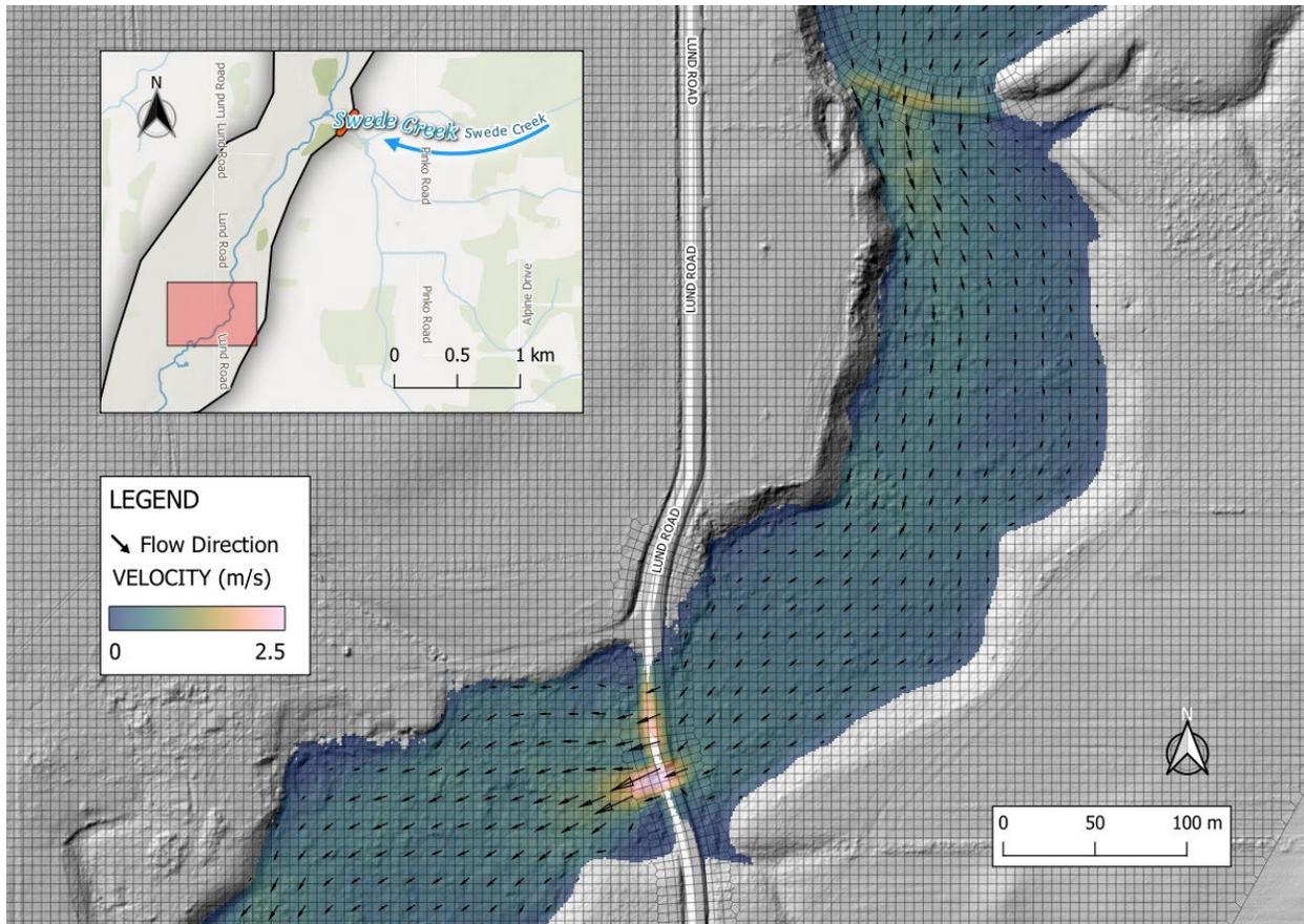
**Figure E-11 Example of the mesh developed for the Tabor Creek at Prince George HEC-RAS model in the vicinity of Lund Road. Modelled flow velocities for the climate-adjusted 200-year flood event are overlaid on the DEM (hillshade). Arrow size is proportional to flow velocity.**
