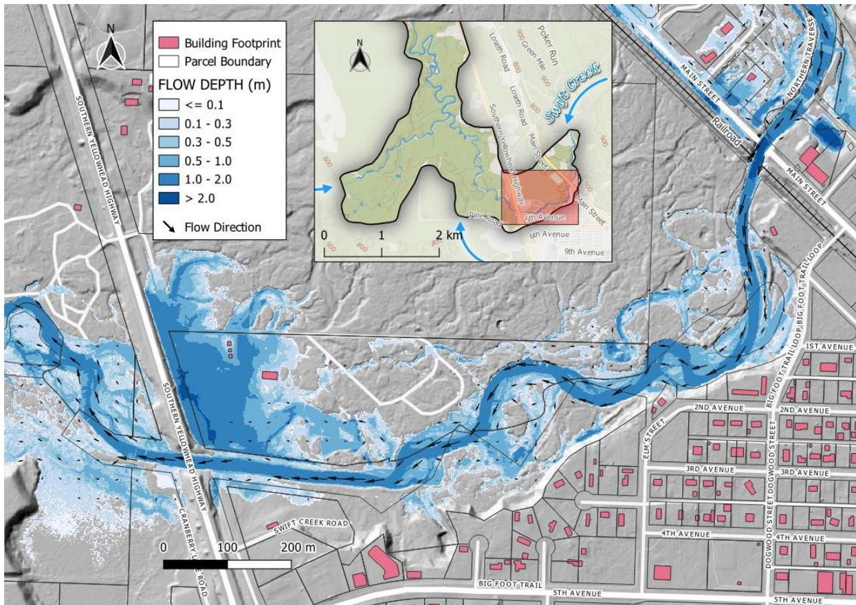
**Figure E-37 Modelled climate-adjusted 200-year (0.5% AEP) Swift Creek flood depth in the vicinity of the Yellowhead Highway, overlaid on the DEM (hillshade). Arrow size is proportional to flow velocity. Building footprints from Microsoft (2023) database (additional buildings likely exist). Parcel boundaries from BC Assessment (2023).**
