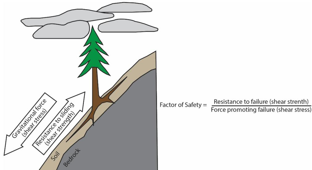
**Figure G-1 Diagram of simplified forces acting on a slope (modified from BCMOF, 1994).**
