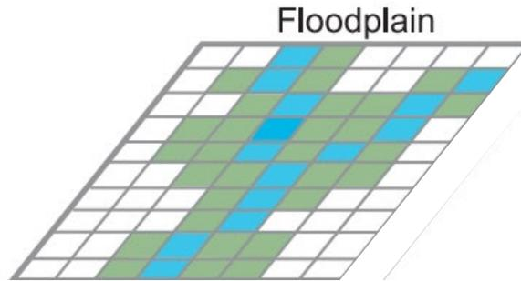
**Figure E-4** Conceptual model of the gridded layer that is derived by defining grids as the 200-year (0.5% AEP) floodplain (green) whose elevations are lower than the corresponding stream network flow levels (blue) (Nardi et al., 2019).
