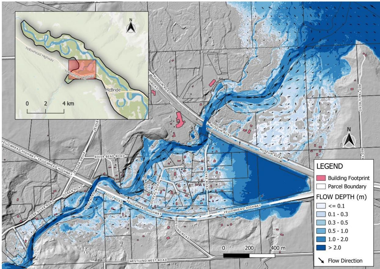
**Figure E-29 Modelled climate-adjusted 200-year (0.5% AEP) flood depth along Dore River, overlaid on the DEM (hillshade). Arrow size is proportional to flow velocity. Building footprints from Microsoft (2023) database (additional buildings likely exist). Parcel boundaries from BC Assessment (2023).**
