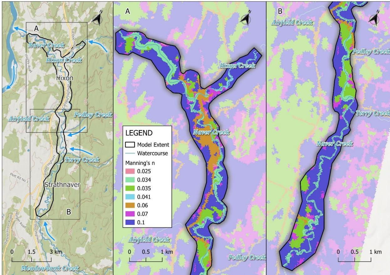
**Figure E-18 Manning's n roughness layer defined for Naver and Hixon Creek at Hixon model.**
