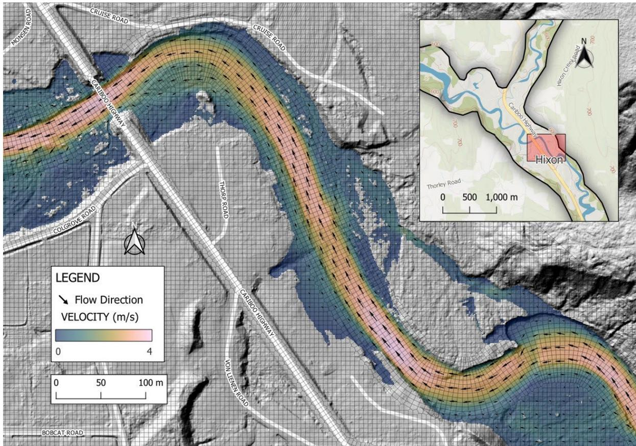
**Figure E-19** Example of the mesh developed for the Naver and Hixon Creek at Hixon HEC-RAS model in the vicinity of the Canyon Creek bridge (Cariboo Highway). Modelled flow velocities for the climate-adjusted 200-year flood event are overlaid on the DEM (hillshade). Arrow size is proportional to flow velocity.
