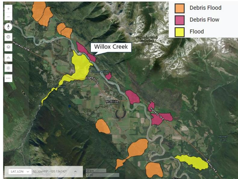
**Figure 4-3 Example of steep creek hazard attributes defined for Willox Creek alluvial fan, north of the Village of McBride.**
