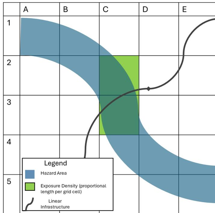
**Figure H-3 Schematic of the hazard exposure calculation logic for polyline-based valued assets.**
