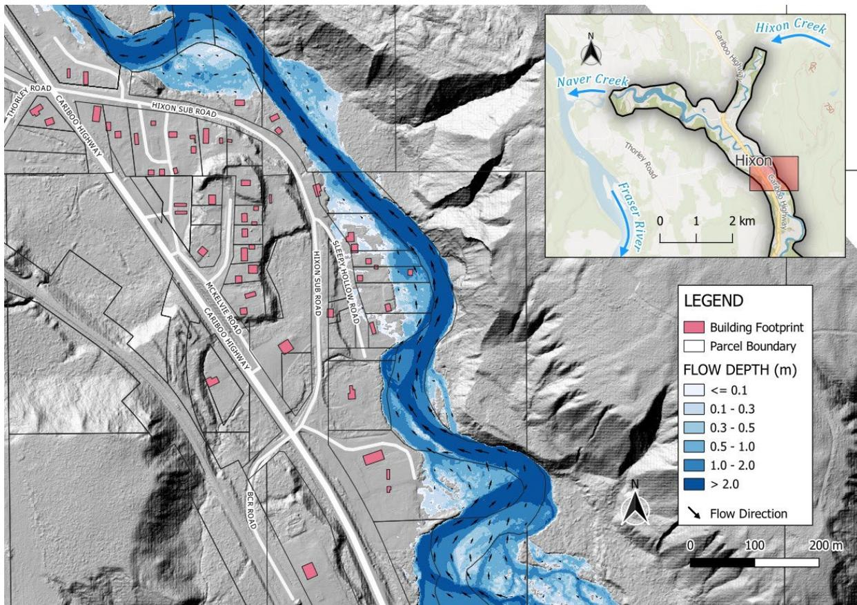
**Figure E-27 Modelled climate-adjusted 200-year (0.5% AEP) Naver Creek flood depth in the vicinity of Hixon Sub Road, overlaid on the DEM (hillshade). Arrow size is proportional to flow velocity. Building footprints from Microsoft (2023) database (additional buildings likely exist). Parcel boundaries from BC Assessment (2023).**
