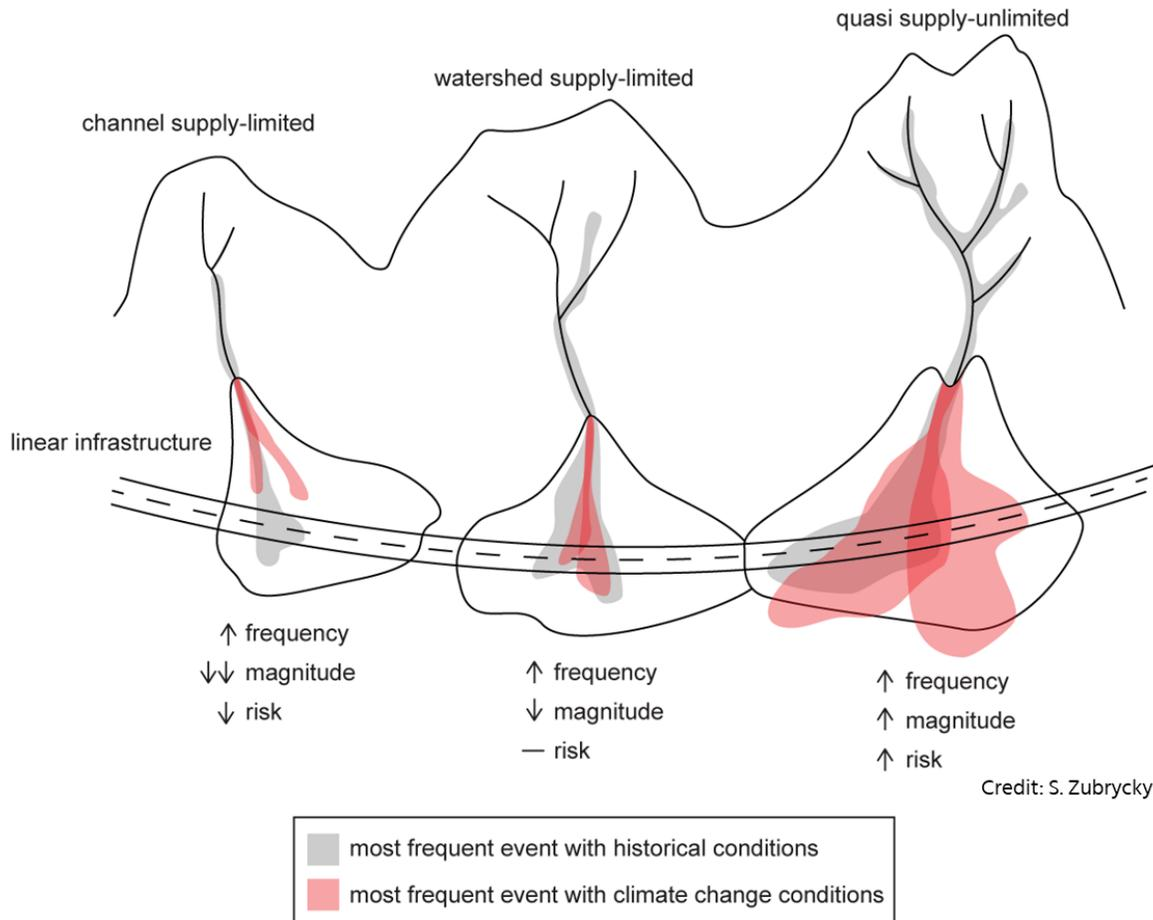
**Figure F-6 Steep creek hazard sensitivity to climate change – supply-limited and supply unlimited basins.**
