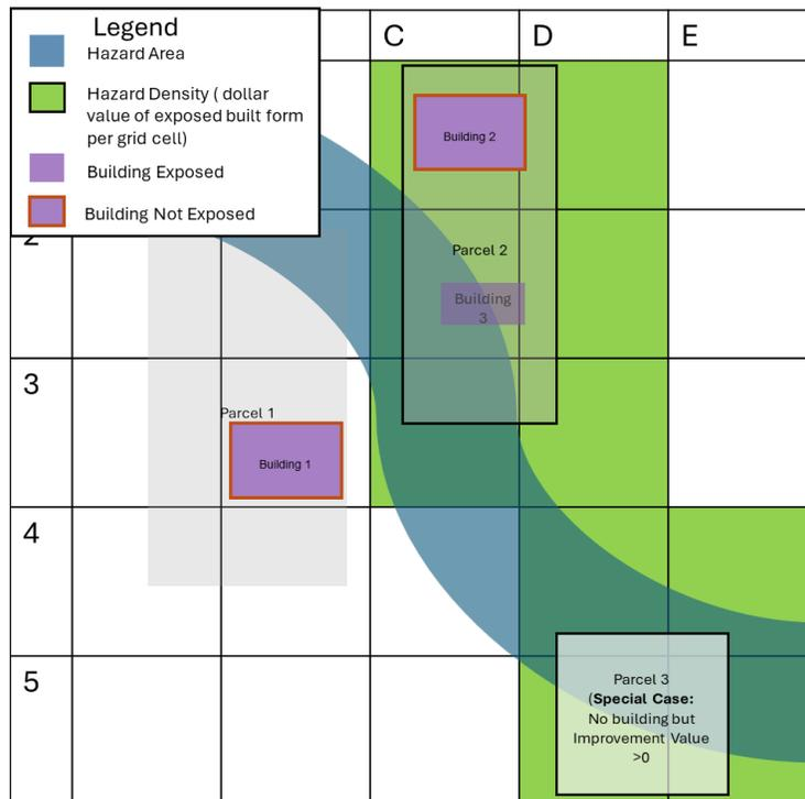
**Figure H-6 Schematic of the hazard exposure calculation logic for cadastral parcels.**
