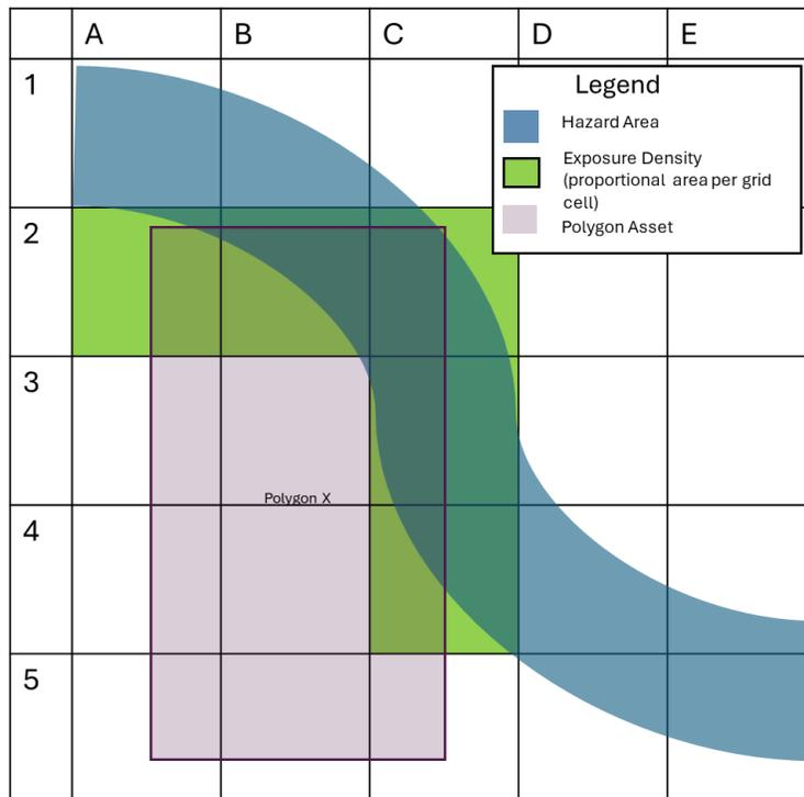
**Figure H-4 Schematic of the hazard exposure calculation logic for polygon-based valued assets.**
