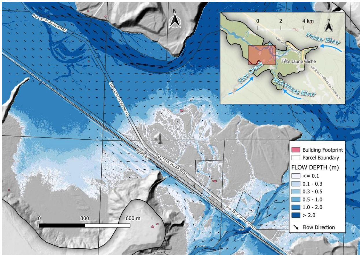
**Figure E-33 Modelled climate-adjusted 200-year (0.5% AEP) flood depth downstream of the confluence of Fraser River and Tête Creek, overlaid on the DEM (hillshade). Arrow size is proportional to flow velocity. Building footprints from Microsoft (2023) database (additional buildings likely exist). Parcel boundaries from BC Assessment (2023).**
