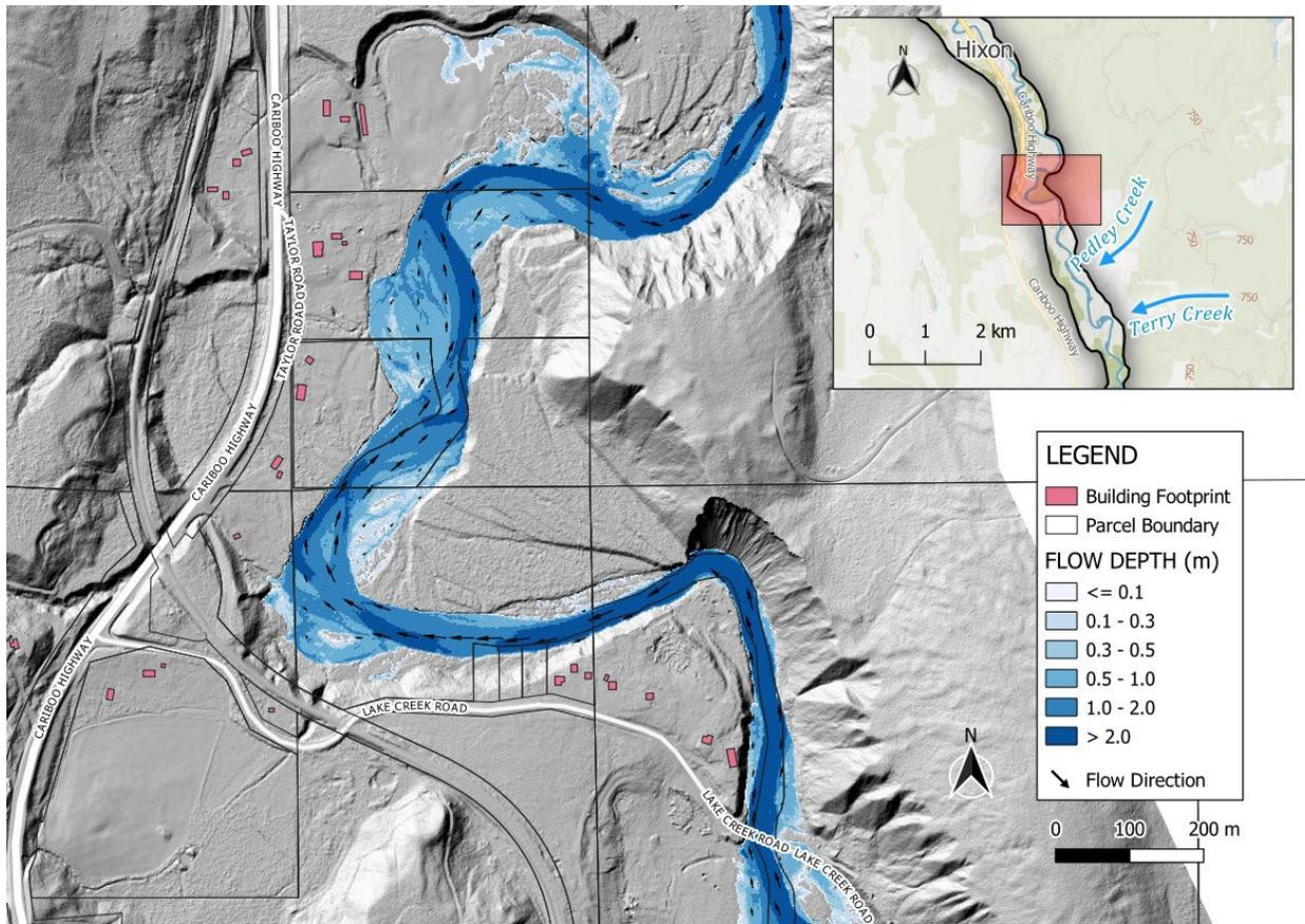
**Figure E-28** Modelled climate-adjusted 200-year (0.5% AEP) Naver Creek flood depth in the vicinity of Lake Creek Road, overlaid on the DEM (hillshade). Arrow size is proportional to flow velocity. Building footprints from Microsoft (2023) database (additional buildings likely exist). Parcel boundaries from BC Assessment (2023).
