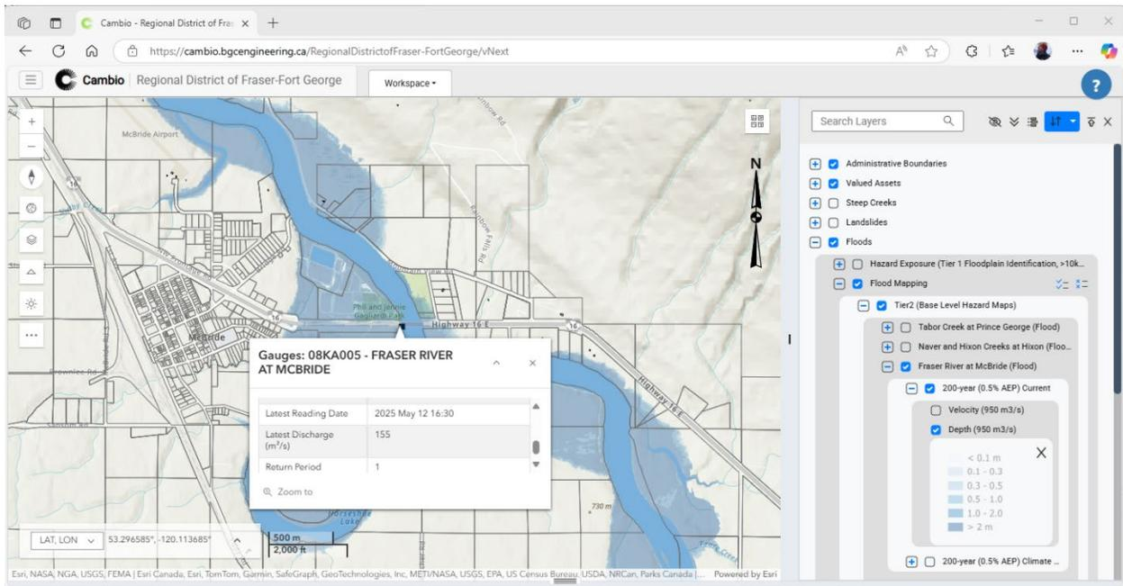
**Figure 8-3 WSC near real-time gauging station on the Fraser River at McBride, within the extent of Tier 2 flood hazard mapping.**
