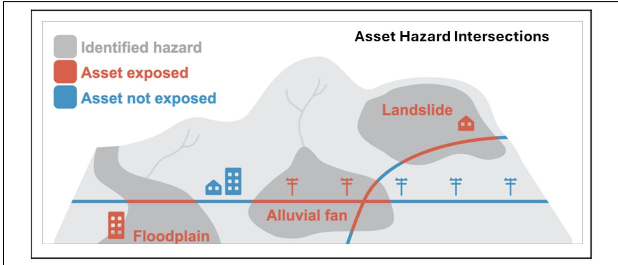
**Figure 5-1** Simplified schematic of the hazard exposure analysis logic where exposure is defined as the spatial overlap between a mapped hazard area and a valued asset.
