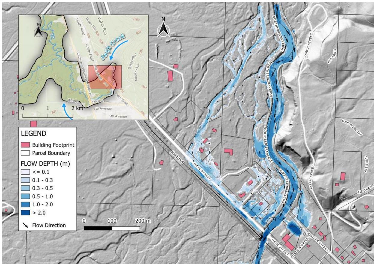
**Figure E-36 Modelled climate-adjusted 200-year (0.5% AEP) Swift Creek flood depth in the vicinity of Main Street, overlaid on the DEM (hillshade). Arrow size is proportional to flow velocity. Building footprints from Microsoft (2023) database (additional buildings likely exist). Parcel boundaries from BC Assessment (2023).**
