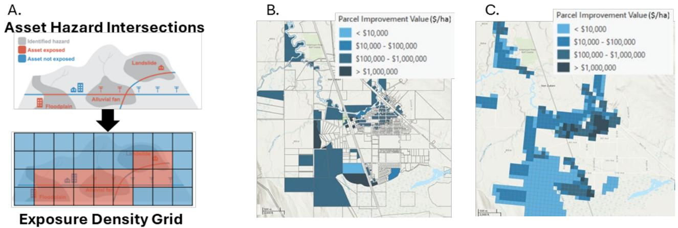
**Figure 5-2 Schematic overview of the hazard exposure analysis workflow and results showing the analysis workflow (left), and outputs, which include hazard asset intersections (middle), and exposure density grid (right)**
