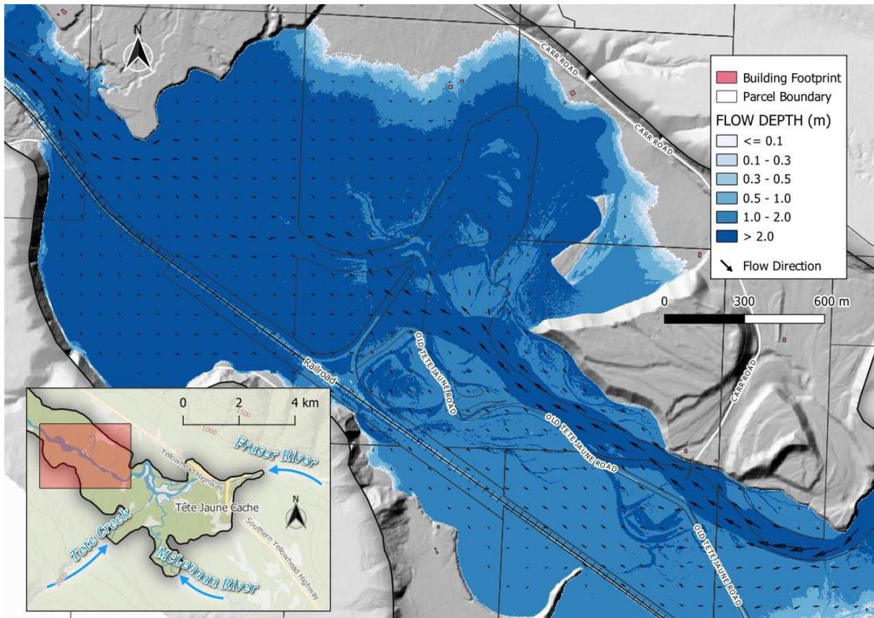
**Figure E-34 Modelled climate-adjusted 200-year (0.5% AEP) Fraser River flood depth in the vicinity of Carr Road, overlaid on the DEM (hillshade). Arrow size is proportional to flow velocity. Building footprints from Microsoft (2023) database (additional buildings likely exist). Parcel boundaries from BC Assessment (2023).**
