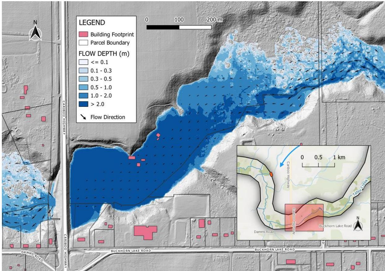
**Figure E-23** Modelled climate-adjusted 200-year (0.5% AEP) Tabor Creek flood depth in the vicinity of Cariboo Highway, overlaid on the DEM (hillshade). Arrow size is proportional to flow velocity. Building footprints from Microsoft (2023) database (additional buildings likely exist). Parcel boundaries from BC Assessment (2023).
