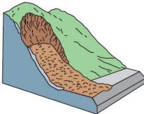
**Figure G-3 Debris avalanche schematic (USGS, 2008).**
