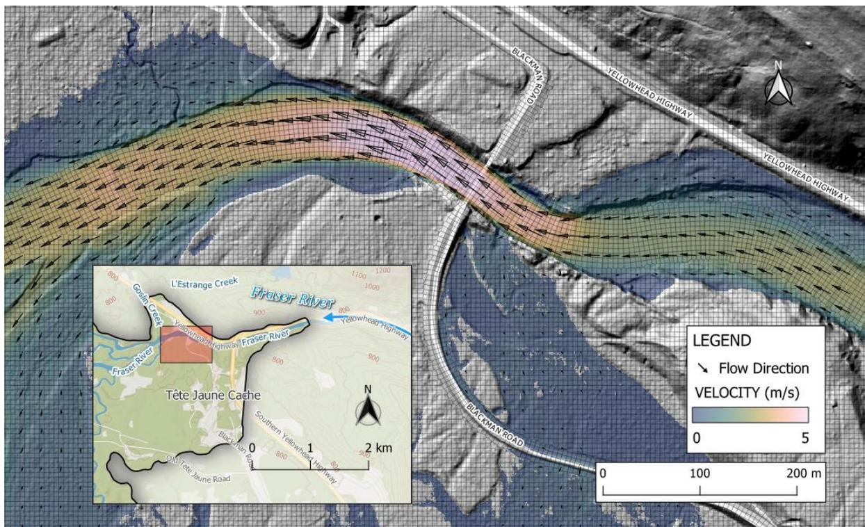
**Figure E-16** Example of the mesh developed for the Fraser River at Tête Jaune Cache HEC-RAS model in the vicinity of the Blackman Road bridge. Modelled flow velocities for the stationary 200-year flood event are overlaid on the DEM (hillshade). Arrow size is proportional to flow velocity.
