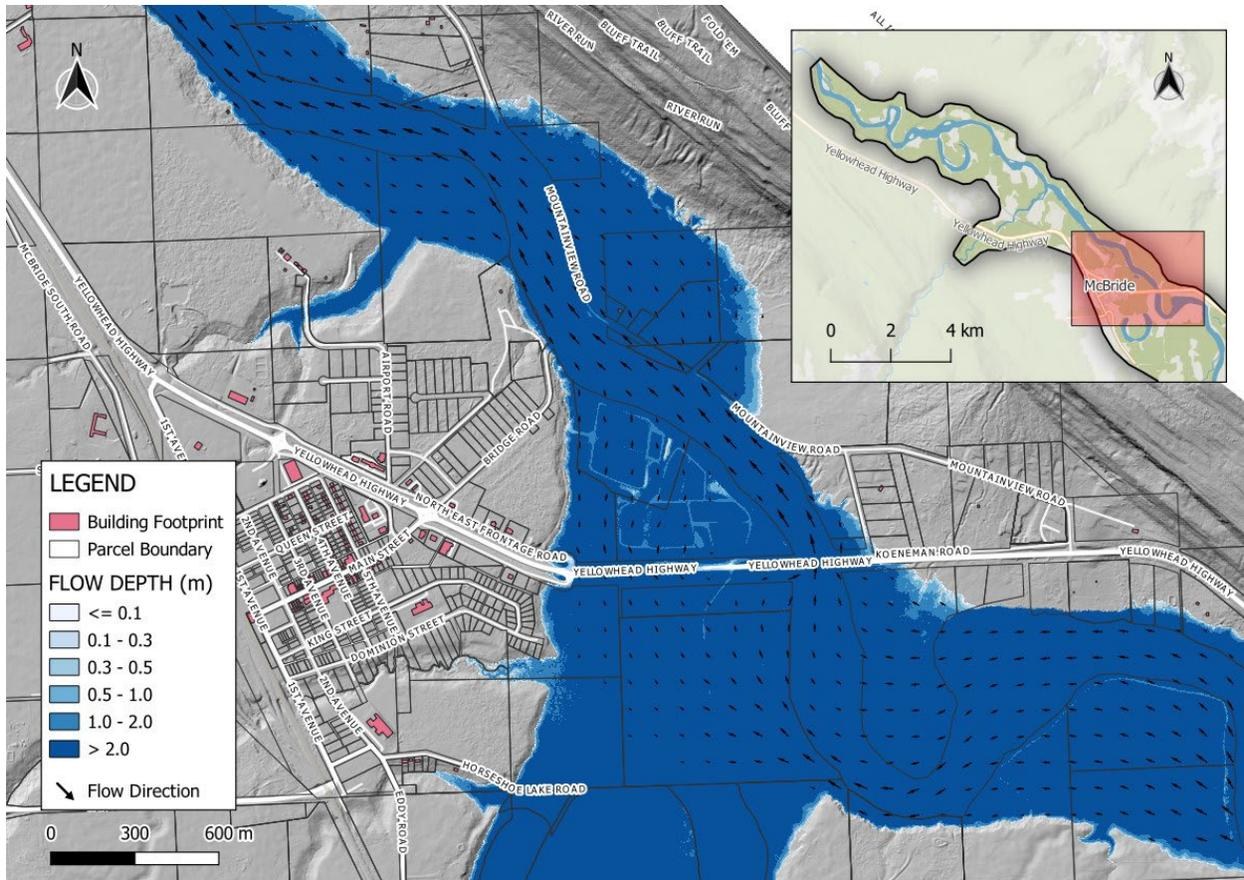
**Figure E-30 Modelled climate-adjusted 200-year (0.5% AEP) flood depth along Fraser River in the vicinity of McBride, overlaid on the DEM (hillshade). Arrow size is proportional to flow velocity. Building footprints from Microsoft (2023) database and OpenStreetMap (additional buildings likely exist). Parcel boundaries from BC Assessment (2023).**
