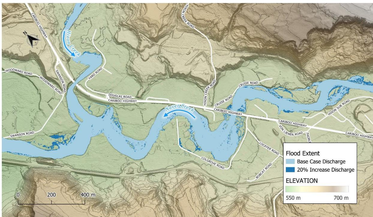
**Figure E-40 Comparison of flood extent between the base case (0.5% AEP) and a scenario with a 20% increase in peak discharge in the vicinity of Naver Creek and Hixon Creek confluence, overlaid on the DEM (coloured multidirectional hillshade). Contour interval is 5 m.**
