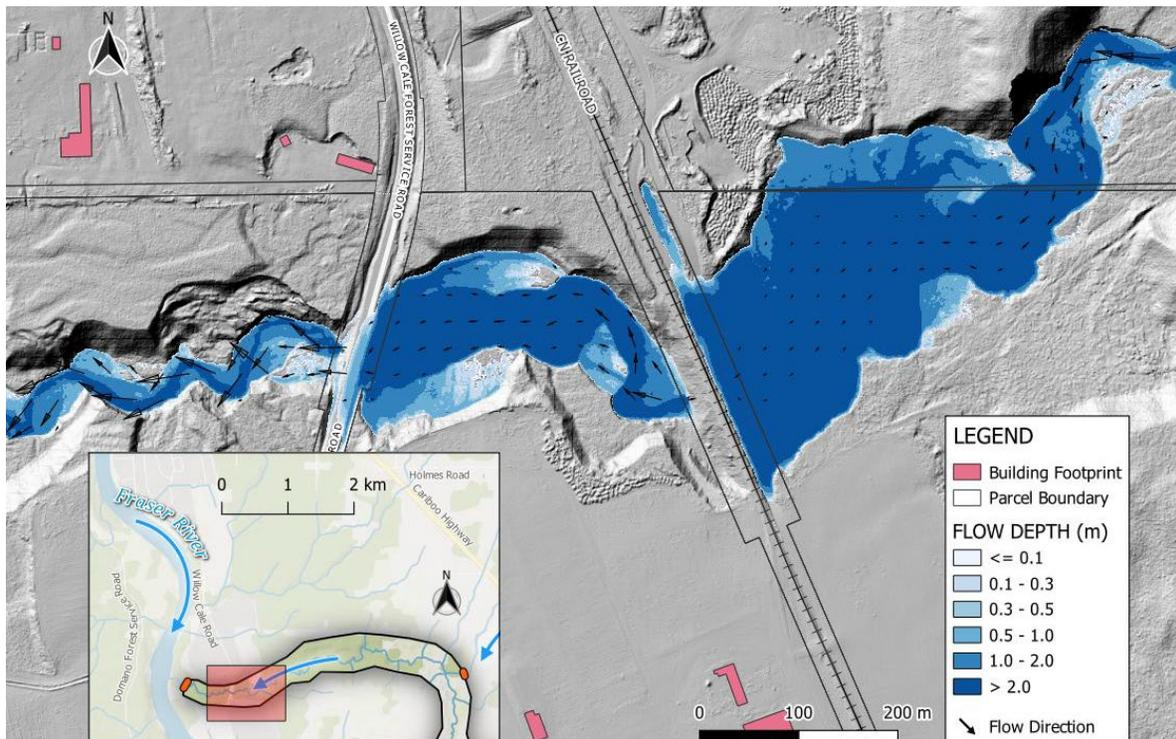
**Figure E-22** Modelled climate-adjusted 200-year (0.5% AEP) Tabor Creek flood depth in the vicinity of Willow Cate FSR, overlaid on the DEM (hillshade). Arrow size is proportional to flow velocity. Building footprints from Microsoft (2023) database (additional buildings likely exist). Parcel boundaries from BC Assessment (2023).
