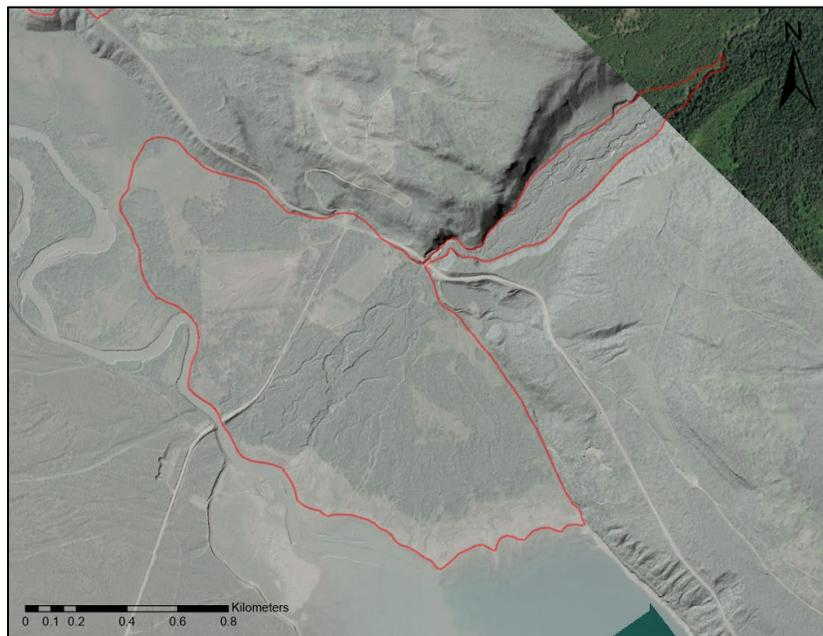
**Figure 4-2 Example alluvial fan boundary, Packsaddle Creek, north end of Kinbasket Lake. Esri imagery overlain by lidar hillshade (Government of BC, 2016).**
