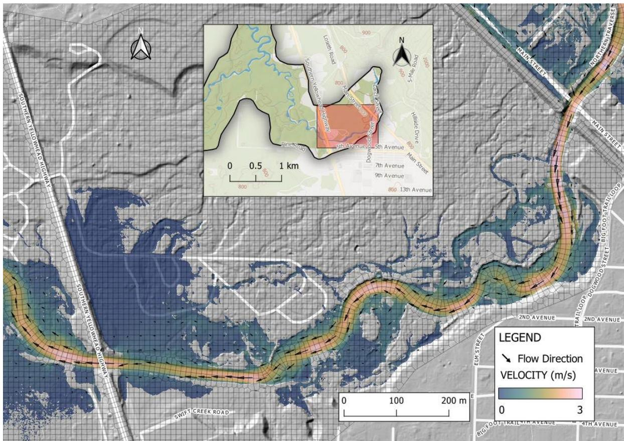
**Figure E-21** Example of the mesh developed for the Swift Creek HEC-RAS model in the vicinity of Valemount. Modelled flow velocities for the climate-adjusted 200-year flood event overlaid on the DEM (hillshade). Arrow size is proportional to flow velocity.
