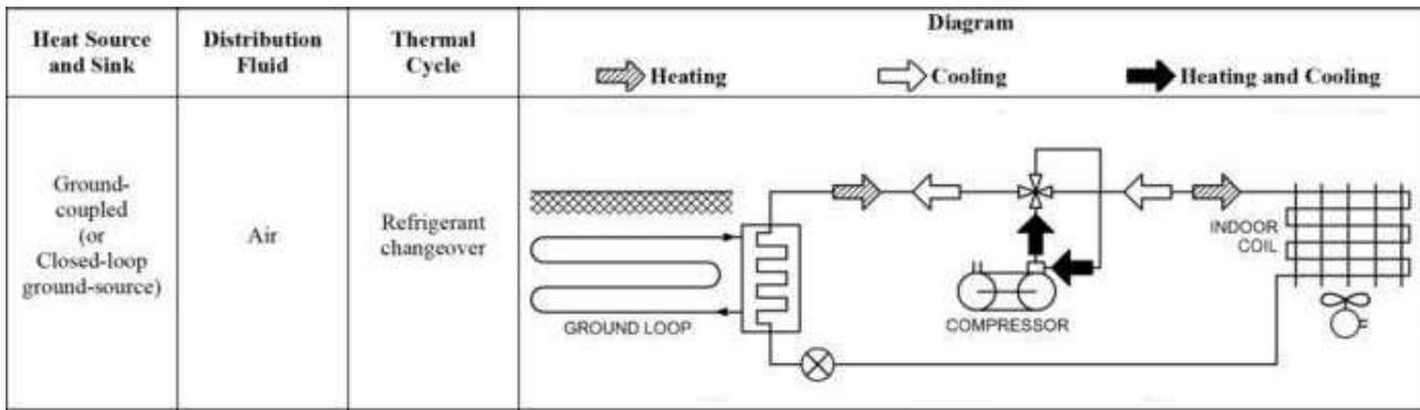
Figure 15 – Ground-Coupled (Closed Loop Ground Source) HP
